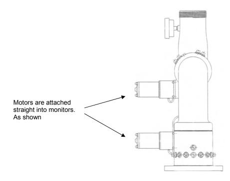
Motor replacement kit is P/N 81453001, if your monitor has the above motor/monitor configuration
