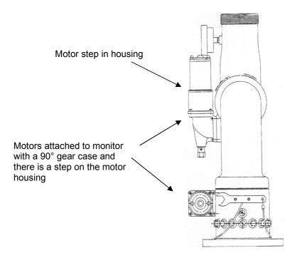
Motor replacement kit is P/N 81301001, if your monitor has the above motor/monitor configuration
