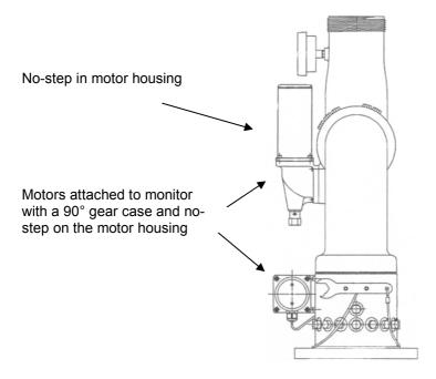
Motor replacement is P/N 81274001, if your monitor has the above motor/monitor configuration. This motor first appeared on monitors built in January 2002 but may appear on older units if the original motor was previously replaced with one of the kits.
