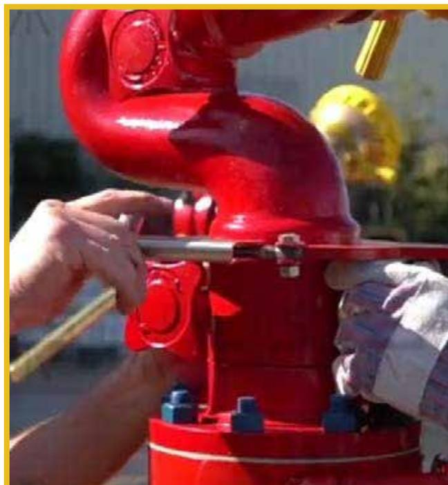
10. It is important to note that due to the nature of the oscillating mechanism, the oscillating arm quick release pull pin must be offset approximately 10 degrees to the left of the center line of the monitor discharge when looking from the monitor to the target. (see Illustration at right)
