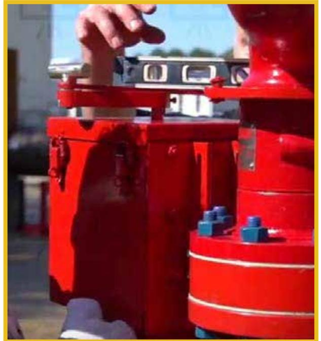
12. Complete the installation by installing the quick release pull pin (A) to connect the connecting link (B) to the swivel clamp(G). Apply a thin coating of GLGI (EP2) grease to holes in the swivel clamp and connecting link prior to installation of the quick release pull pin.
