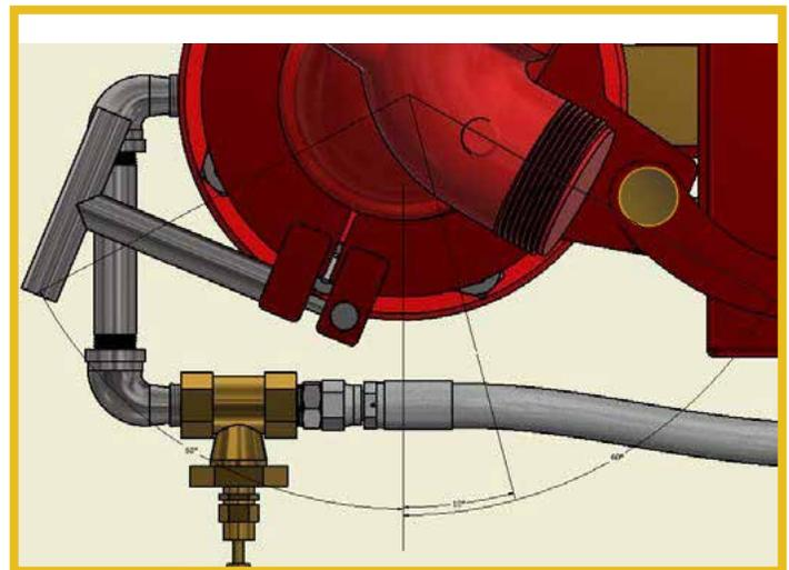
11. Next, the elevation of the water turbine must be adjusted so that the connecting link is level.
