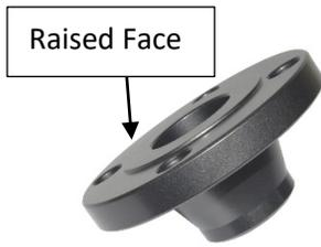
Bolted pipe flanges come in several styles. The two most common styles are flat faced [FF] and raised face [RF]. Pictured at the left is an RF weld neck flange. It is easily identifiable by the raised annular ring around the perimeter of the flow area. A FF flange looks similar but without the raised portion.
